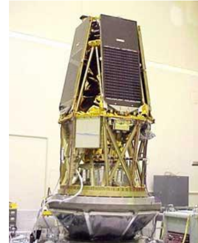
HESSI after repair. The test in March 2000 that caused the failure was lateral, on a slip table.
