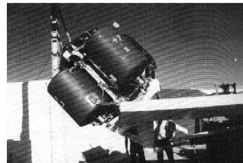
Propulsion module on Sandia Labs centrifuge, Fig. 11.8 from Ref. 1 (SSAM)
