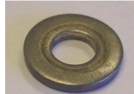
NAS1149C0363R (300-series CRES) washer that yielded under a preloaded A-286 socket-head cap screw
